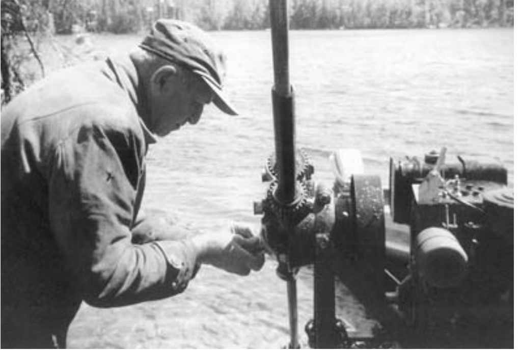
Hanson's Exray diamond drill, which could reach down to 150 feet, was in great demand in the Flin Flon area.
