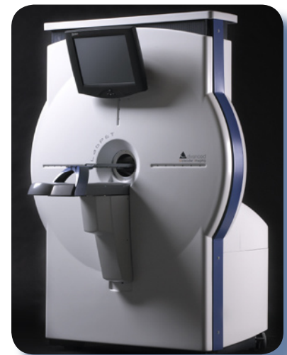
LabPET™ Small Animal Scanner commercialized by AMI Inc. Image courtesy of Roger Lecomte
