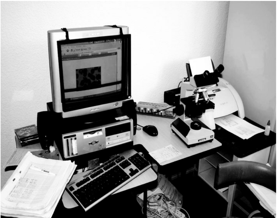
Figure 18.4 Primary care site in Macas. Computers are connected via a local area network (LAN). The unit shown is stationed in the clinic's laboratory, and can import microscopic images into the EHR, via an eyepiece camera
