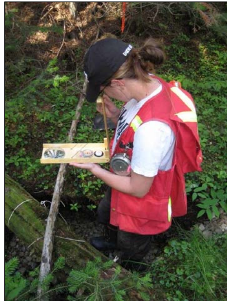
Figure 3. Shade measurement using the spherical angular canopy densiometer at one point along a small stream control reach, August 2008.
