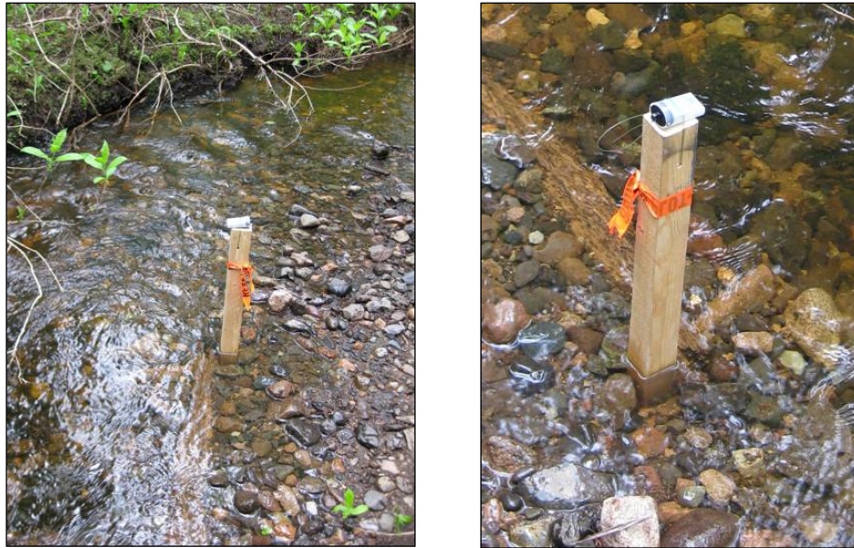
Figure 5. Field deployment of Hobo Pendant Logger on top of a stake approximately 50 cm above the stream surface, August 2008.
