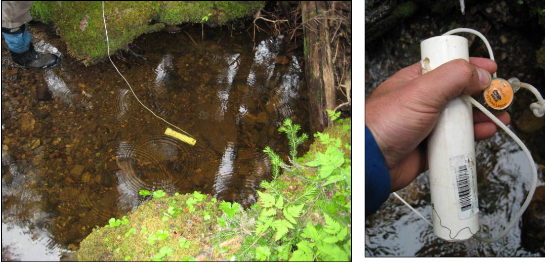
Figure 6. Field deployment of Tidbit™ temperature logger and solar shield in a pool, August 2008.
