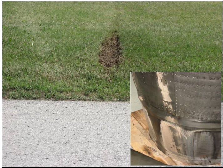
Photo 2. Ground scar from number 2 engine tailpipe (inset)
