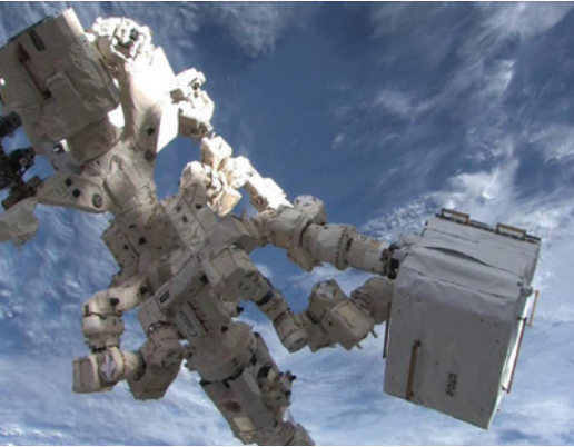
Dextre, the Canadian Space Agency's robotic handyman, ferries cargo from the Kounotori2 cargo ship to the International Space Station in February 2011. (Credit: NASA)
