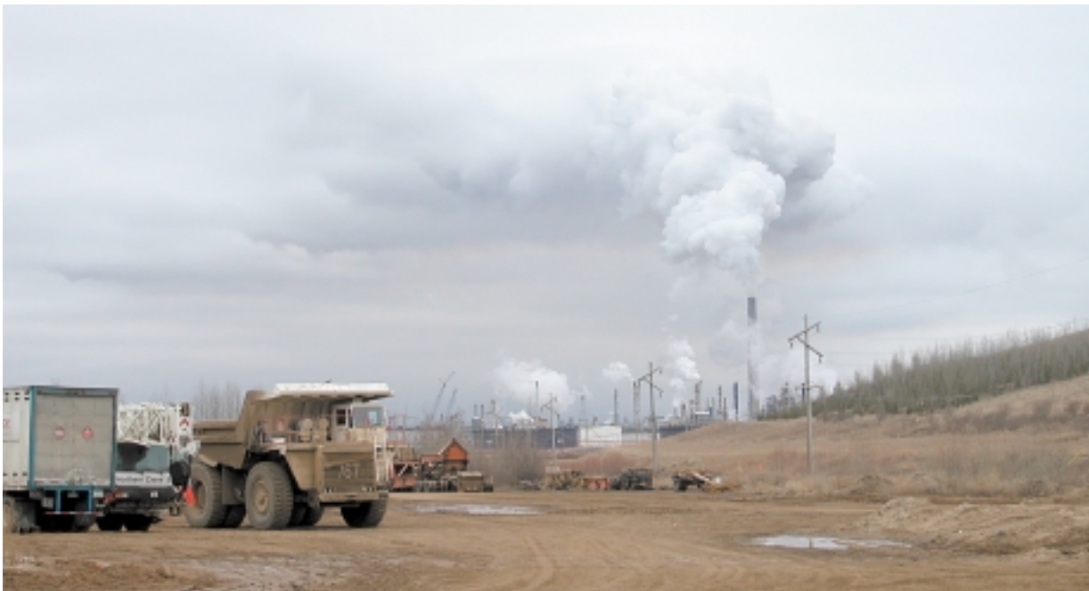
▲ Oil sands mine truck fleets are a major source of NO x emissions.
