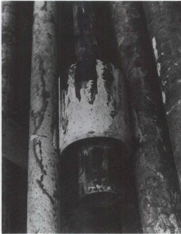
FIGURE 10 Ocean Ranger hang-off tool. The large diameter steel bottom section is designed to rest on the pipe rams of the BOP stack.
