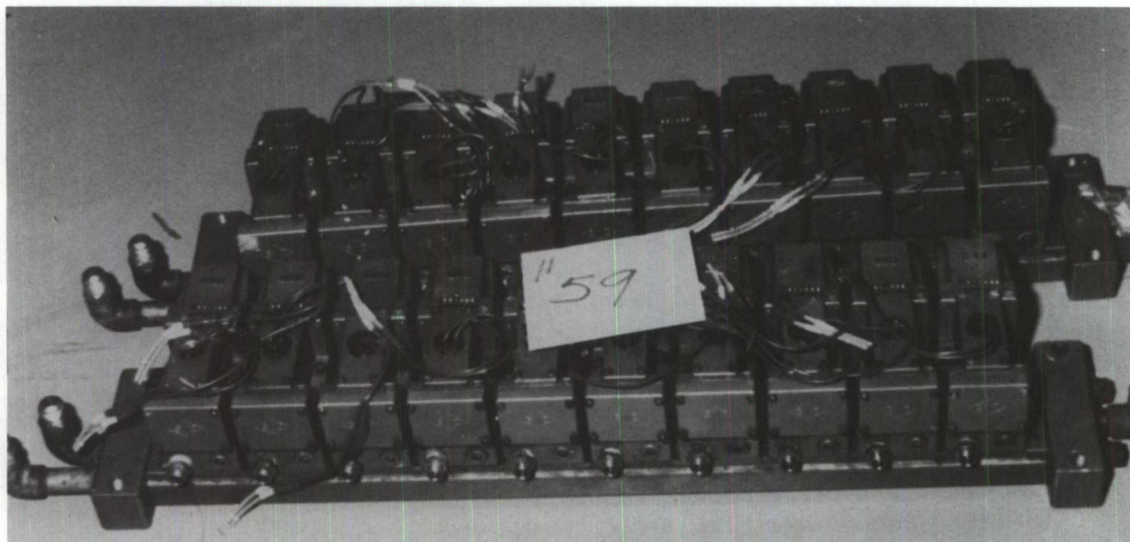
PHOTOS 1-3 The six solenoid valve banks as received. The manifold intake and exhaust ends are indicated in the centre photograph.
