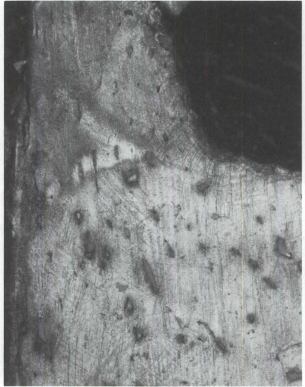
PHOTO 17 Porthole No. 4 locking ring cross section showing high concentration of deformation slip lines around the base of the protruding lip.
