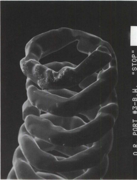
PHOTO 6 Smooth fracture surface of port #3 ballast water stop.
