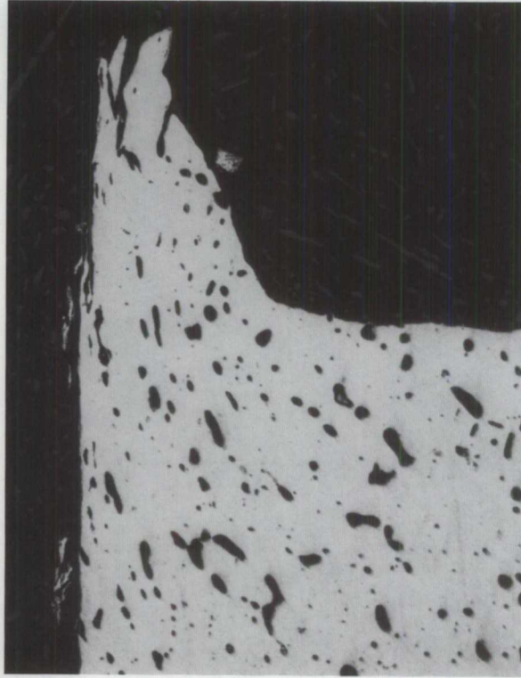
PHOTO 11 Cross section of retaining ring from porthole No. 4 shows similar protruding lip.
