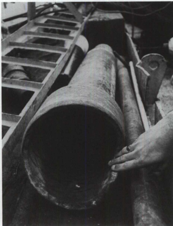
FIGURE 7 Mill used to grind down the sheared end of the drill pipe.
