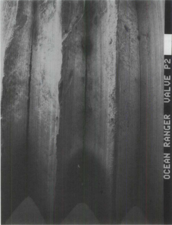
PHOTO 17 SEM photograph showing cracks observed in the thread roots of a failed actuator rod. This was typical for all 14 broken actuator rods examined.
