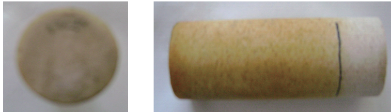
Figure 6 Condition of Core Edge Pollution and Leading Advance (Effective Permeability is 410mD)
