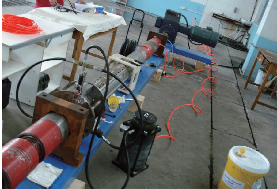
Figure 5 RSM Tool in Test Stand with Load Ring and Rotation Sensor
