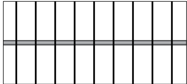
Figure 2 Schematic of a Homogeneous Multi-Fractured Horizontal Well Completion
