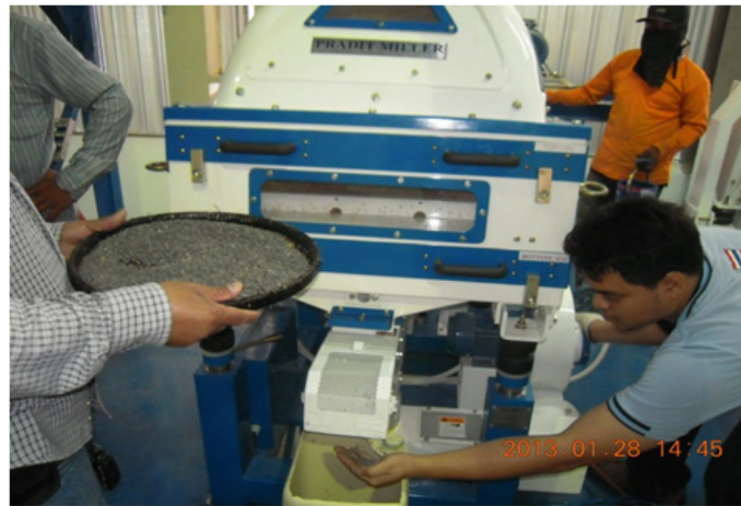
Figure 6. A machine for removing grit from the rice
