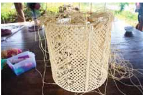
Figure 4. Make weaves as designed to cover every side of the frame in even spacing and patterns
