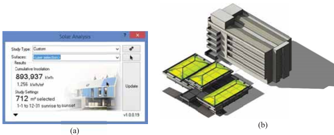
Figure 11. (a) Solar Analysis results of the 0°CW at 6-meter distance (b) gradient colors of the ranges between the minimum cumulative insolation (purple) and the maximum (bright green) on the analyzed surfaces
