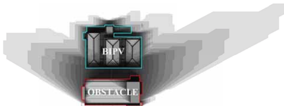
Figure 6. An illustration of a shadow range from 8.00 am to 5.00 pm on winter solstice, demonstrates a common problem that PV system designers may encounter to optimize the rooftop PV system deployment.
