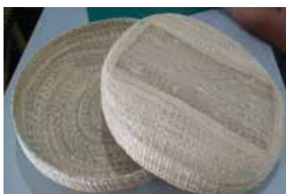
Figure 13. After interlacing and taking out from the archetype before fixing with leather.
