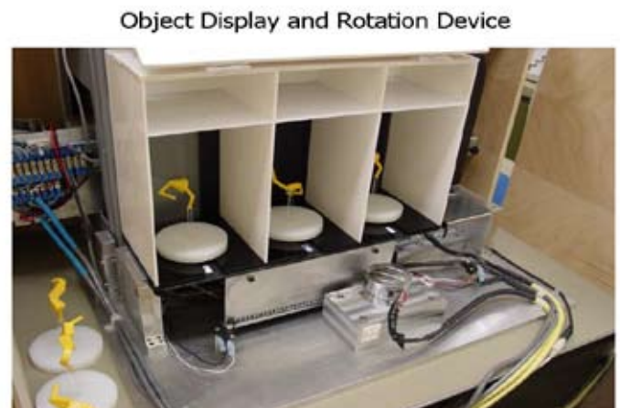
Figure 12. Back view of apparatus used to display and rotate actual 3-D objects. See Friedman et al., 2003 for details.
