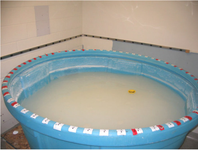
Figure 1. An image of a Morris water maze created from a round (2 m diameter) cattle trough. The position of the hidden platform is revealed by a light colored disk in the right portion of the pool. The markers on the perimeter of the maze indicate a coordinate system for placing multiple landmarks. Photo courtesy of Brett M. Gibson.
