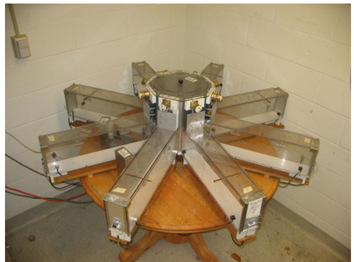
Figure 2. An image of an enclosed and fully automated 8-arm radial maze. Entries between the arms and central chamber are recorded using a system of photocells. Water can be dispensed in the distal ends of the arm by a pump and used as a reward for correct responses. Plexiglas guillotine doors between the arms and central chamber can be raised or lowered by a computer controlling the session. Photo courtesy of Brett M. Gibson.
