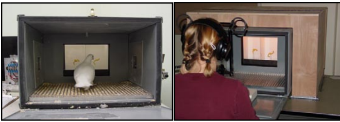
Figure 13. Front view of the object rotation apparatus as used for pigeons and humans. From Friedman et al., 2003.
