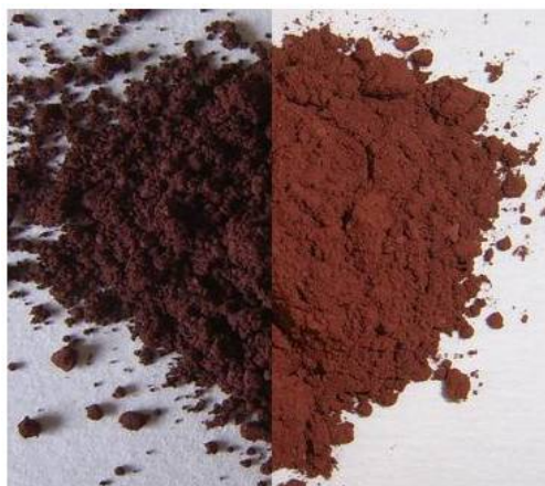
Figure 4. The figure of uncoated red phosphorus and red phosphorus microcapsule
