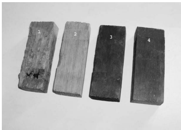
Figure 7. Wood samples after one year of graveyard test
