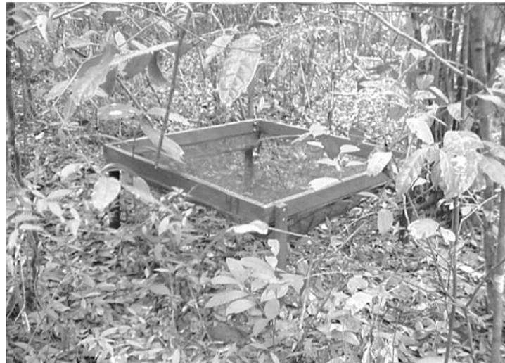
Figure 2. Litter collector in control treatment, installed 30 cm above the soil surface, in successional forest, Castanhal/PA
