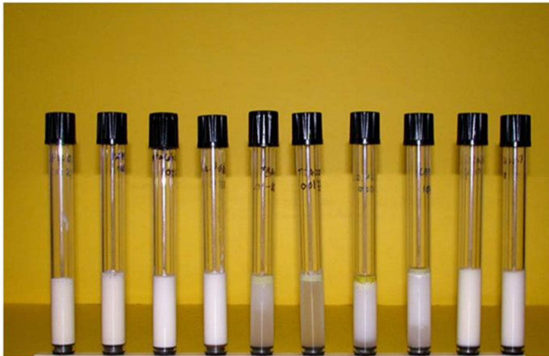
SPI/Oil SPI/Oil STA/Oil STA/Oil TRA/Oil TRA/Oil CAR/Oil CAR/Oil GA/Oil GA/Oil 10/20% 10/10% 10/20% 10/10% .025/10% .025/5% 0.1/10% 0.1/5% 10/20% 10/10% GA: gum arabic; CAR: carrageenan; TRA: tragacanth; STA: starch; SPI: soy protein isolate
