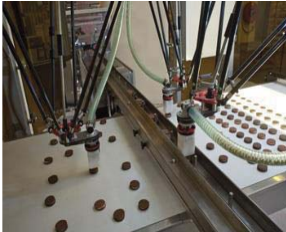
Figure 7a. Delta robot (In Cookie Factory)
