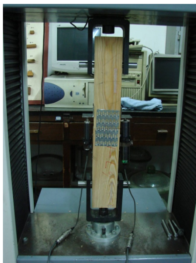
Figure 1. Experimental set up utilized in the tensile tests performed on MPC joint
