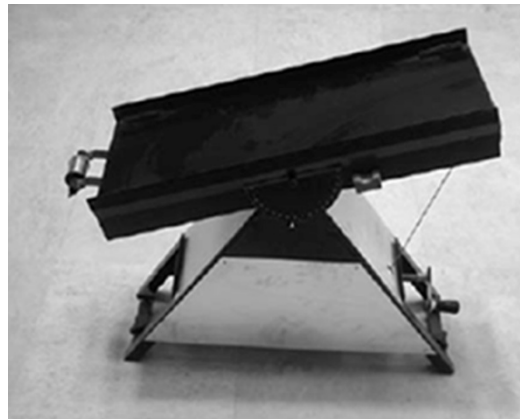
Figure 2. Apparatus to determine coefficient of static friction
