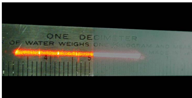
Figure 5. Reflection of the laser line along a stainless steel scale bar illustrating the necessity to coat reflective objects. The left half of the bar was left uncoated while the right side was lightly dusted with ammonium chloride.
