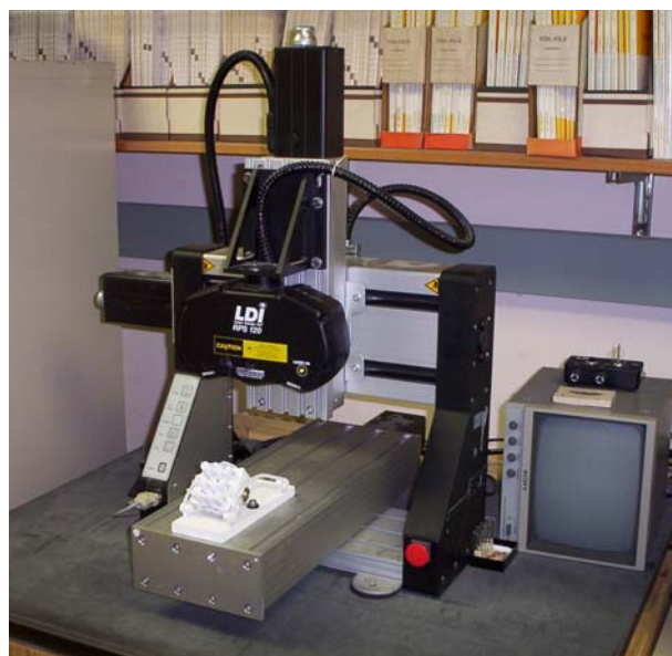
Figure 1. Laser scanning system consisting of a Laser Design Inc. RPS 120 probe mounted on an ISEL Automation computer numerical control (CNC) gantry unit.
