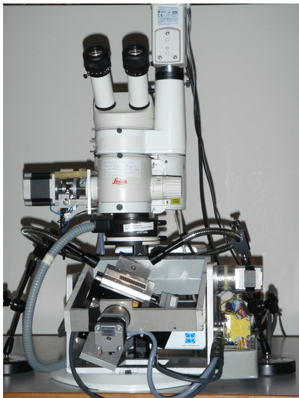
Figure 1. Motorized binocular and 4-axis gliding and tilting stage of AMOR (Automated Measurement system for shell mORphology).
