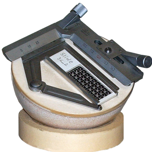
Figure 2. Hemispherical stage. Microfossils are mounted on a standard multisquared faunal slide, one specimen per field. The slide is fixed on a hemispherical body of polystyrene that sits on a ring-shaped basin.
