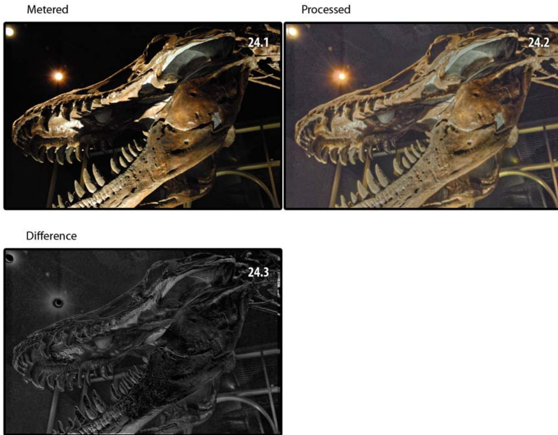
FIGURE 24. High ISO noise in low light. 24.1 original metered exposure, 24.2 tonemapped HDR image, 24.3 difference map as in Figure 6.
