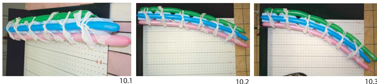
Figure 10. Experiment E8. The possible option to move the chain beam by unilateral pressure increase of one pneumatic body in a triple system of pneumatic bodies was studied. 10.1. At a pressure of 0.15 bar, the chain beam lay with its panel in a horizontal plane, so that the belt joints stood vertical. 10.2. and 10.3. Increasing the pressure in the right balloon to 0.25 bar resulted in a curvature bi of 405 mm of the whole beam to the right side.
