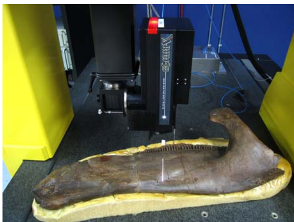
Figure 4. The Arios 3D laser scanner scanning dentary of Edmontosaurus , CMN 2289.
