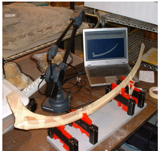
FIGURE 7. Digitizing a Brachylophosaurus canadensis rib (JRDI 200, length 1048 mm). Note the extensive markings on the bone. The finished 3D file is visible on the laptop screen.
