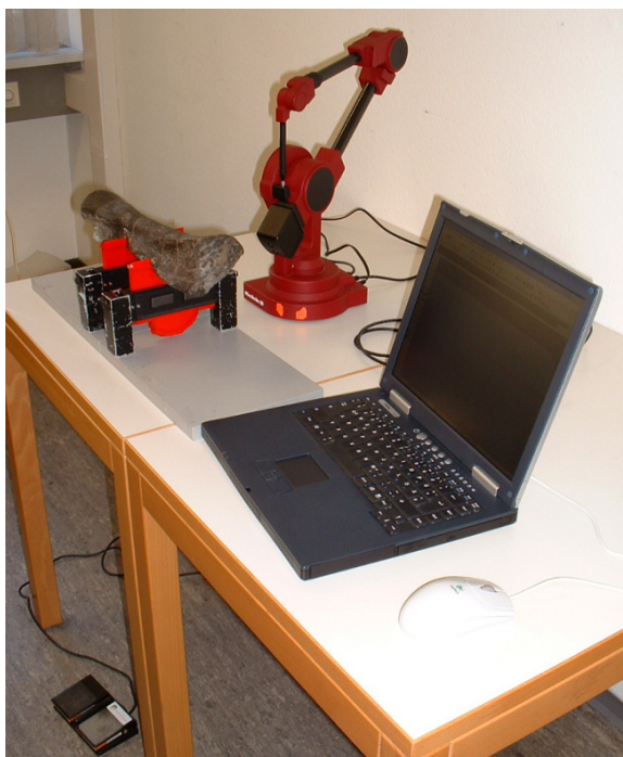
FIGURE 1. Typical setup for digitizing: laptop, digitizer, and fossil holder. Note the position of the digitizer close to the fossil and away from the operator, so that the tip can be pulled instead of pushed.
