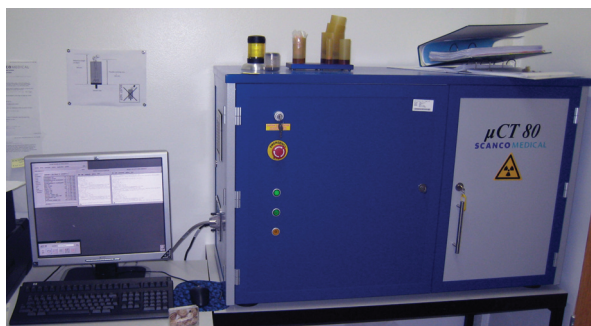
FIGURE 4. Micro-computed tomograph Scanco® micro-CT 80 of the Anthropological Institute (University of Zürich) enabling acquisition of digital three-dimensional data of gastropod shells.
