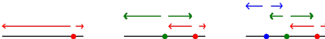
Figure 5: The path-ordered integral is depicted as a power series over integrals. The first term (not drawn) is the identity. The second term is the integral of A_t (depicted as a bullet on the interval) over all t from the right to the left (the orientation goes from right to left). The third term is the integral of A_t A_s over the interval but keeping earlier operators to the right. This is drawn by showing the bullet on the right being able to move along the interval provided it stays behind the bullet to its left. The fourth term involves three operators. Higher terms are not drawn. All terms are summed with appropriate factors.
