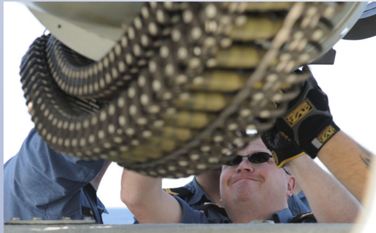
Loading 20mm ammunition into a Royal Canadian Navy Close in Weapon System (CIWS) (Photo Source: Department of National Defence)
