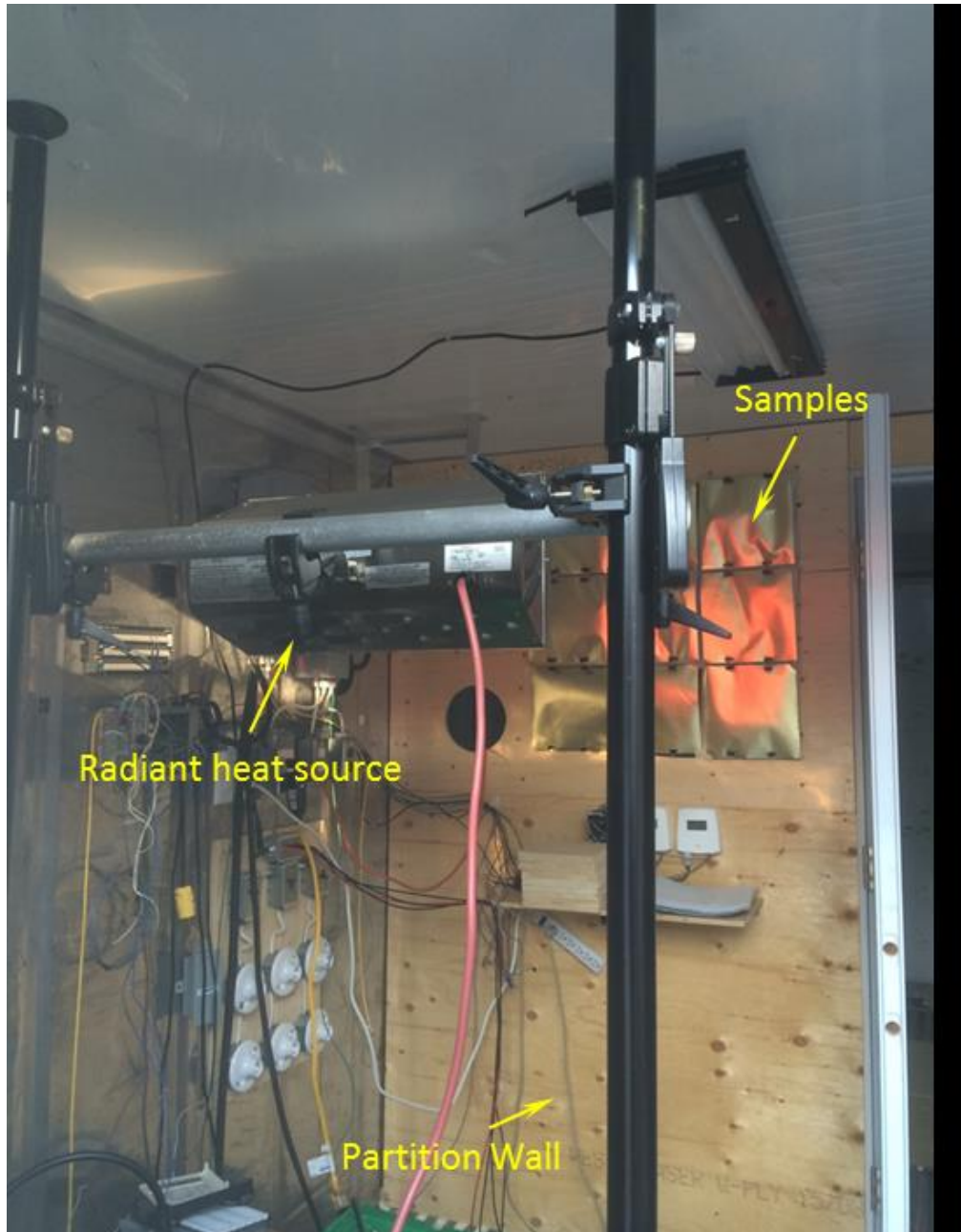
Figure 4: TEST 3 – Set-up for Testing of Layer Configurations
