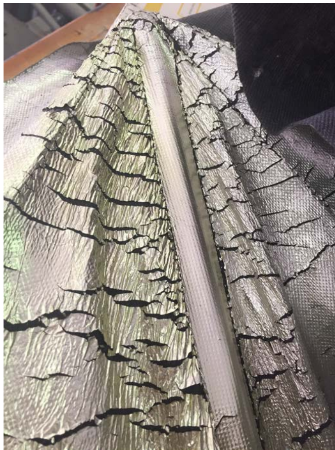
Figure 7: TEST 1 – Splitting of the Heat Reflective Layer (Tensile Stress)
