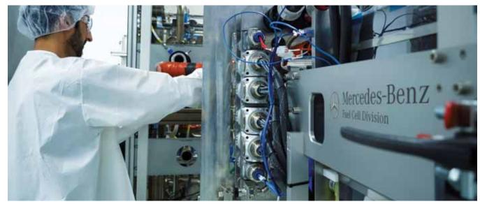
Factory acceptions test with operator at Mercedes Benz Fuel Cell Stack Production (Burnaby, British Columbia). Photo courtesy of Mercedes-Benz
