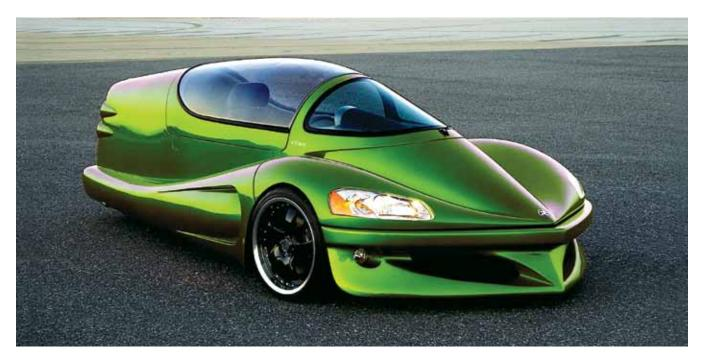
The eVaro car, developed in Canada, is a three-wheeled electric sports car that can achieve speeds of up to 210 km/h and travel 200 km between charges.
