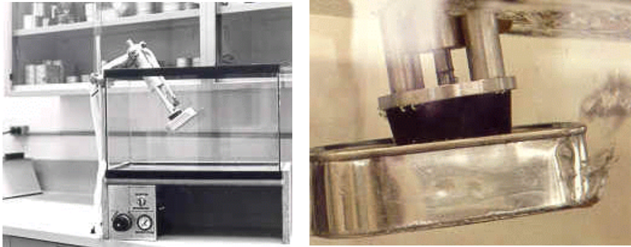
Figure 4.2.2 - Pressure Testing Device
