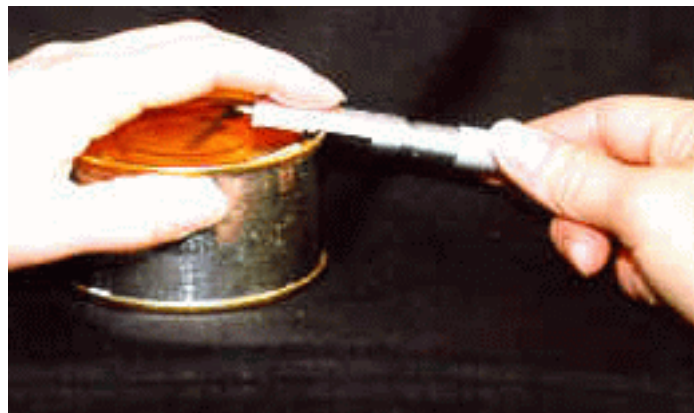
Figure 4.1.2.d - Seam Thickness Measurement
