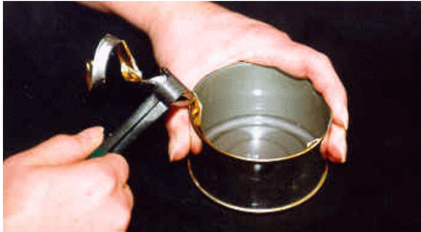
Figure 4.1.3.b - Removing Can End
