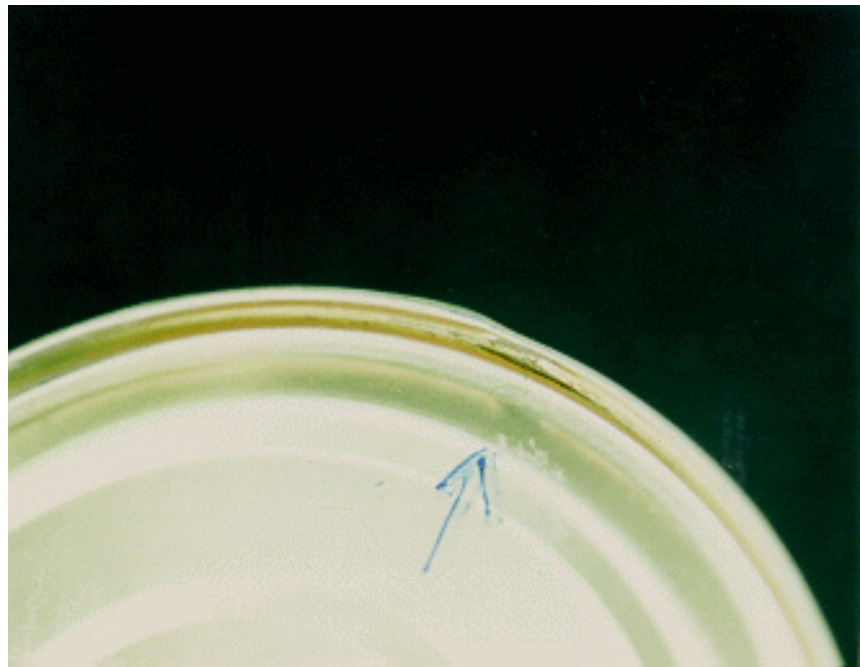
Countersink wall radius showing scuffing caused by chuck slipping
