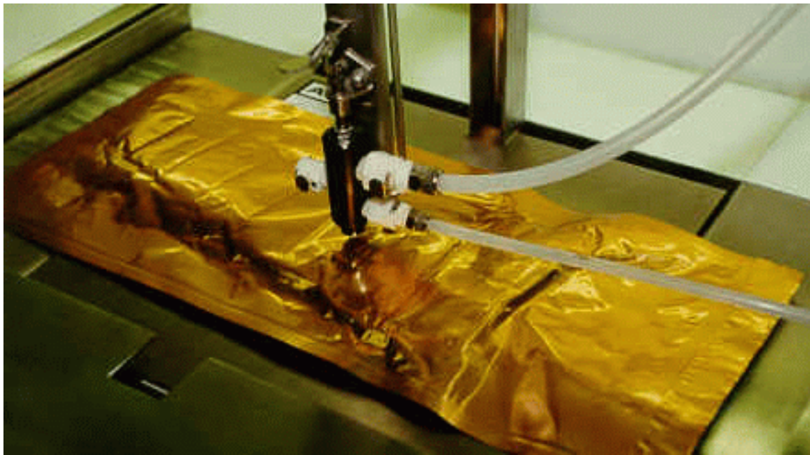
Figure 4.3 Internal Burst Test Equipment - 4-sided tester Pouches are restrained between two plates, shown in the open position (top picture)
