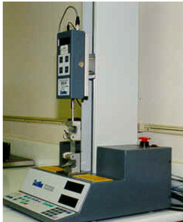
Figure 4.6 Tensile Test Equipment Showing Sample being Tested
