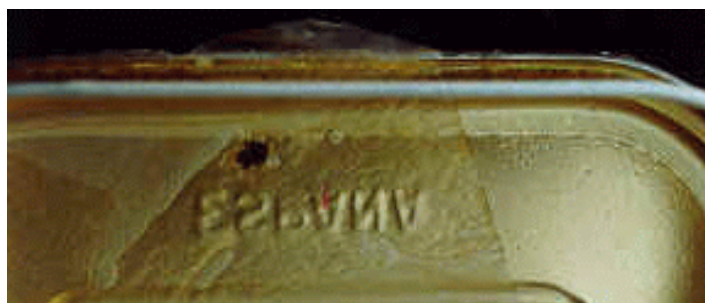
PARCHMENT PAPER FORMED INTO DOUBLE SEAM.
