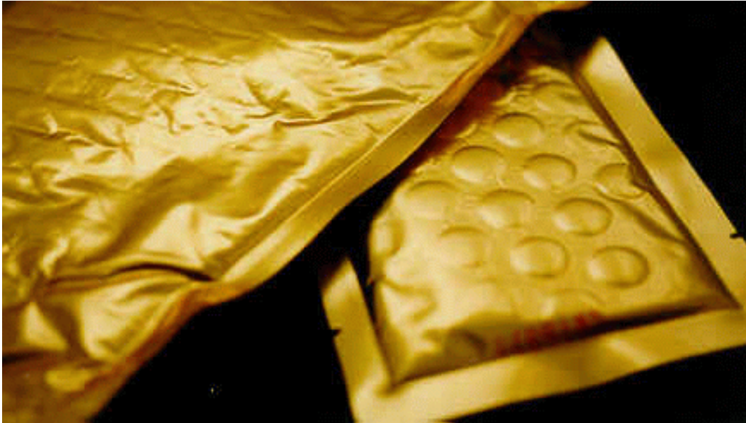
Impressions of retort rack pattern on pouch body
