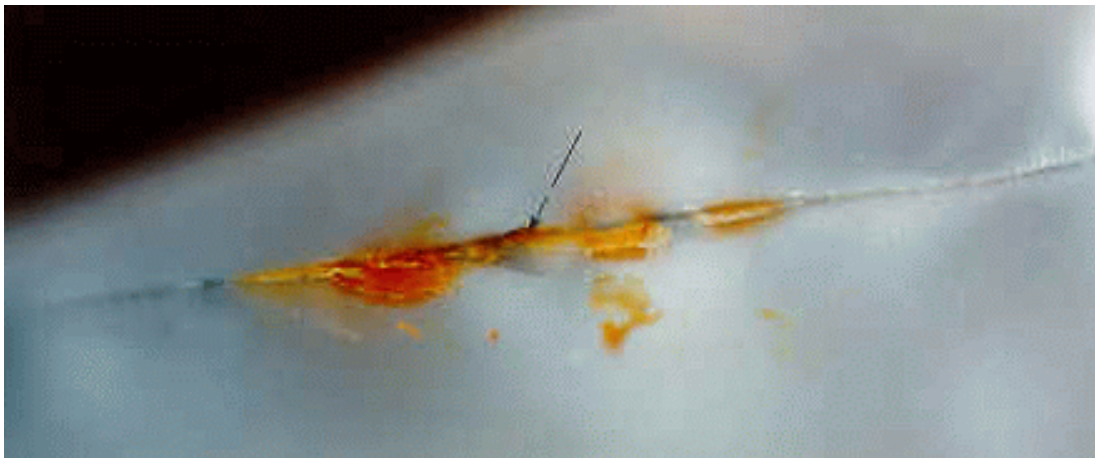
View of Channel Leaker from Inside of Pouch (arrow indicates channel)
