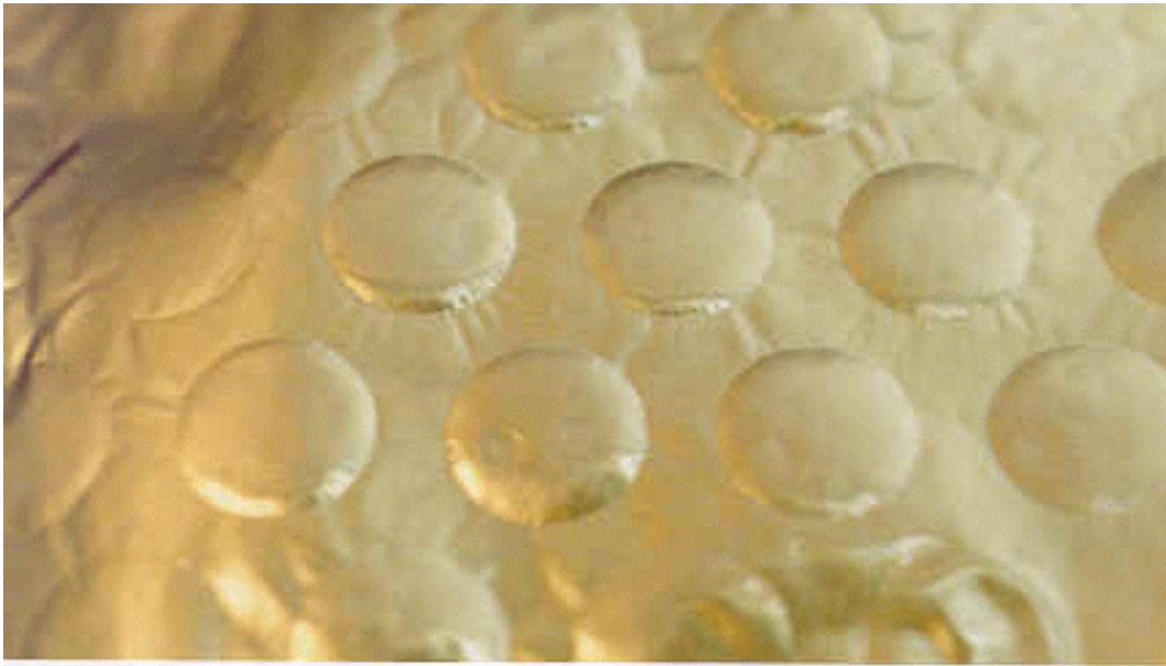
Close-up of impression on surface of pouch body - Waffling
