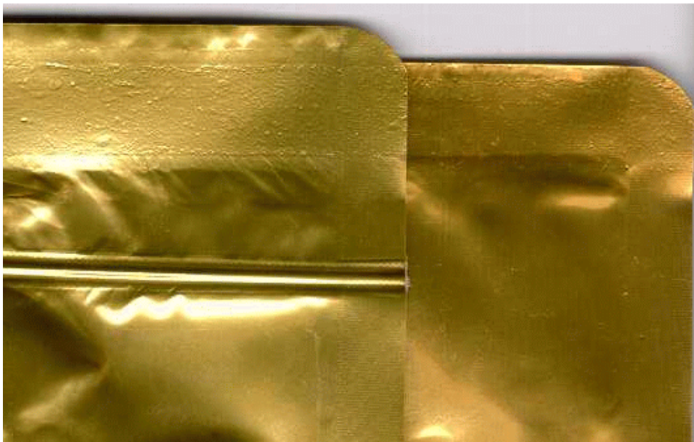
Pouch on Left with Both Primary and Cosmetic Seals; Pouch on Right with Cosmetic Seal Only
