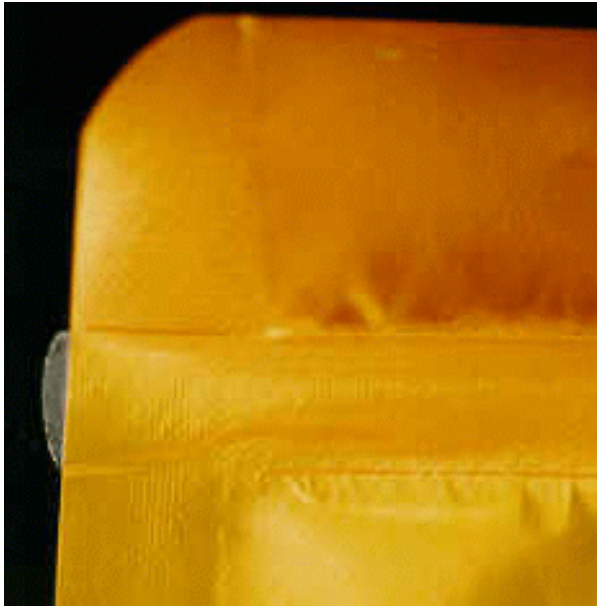
Normal sealing bar impression
